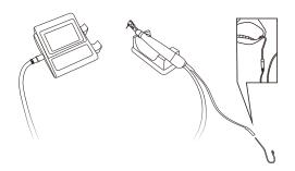
M4: With the function of root canal measuring root canal expanded, after the root canal file into the root canal, the file started forward. After the file arrives the district of root canal stenosis, it begins to rotate slowly, and then automatically reverse when arrived at the apices of the setting position. It restores the original speed operation after leave narrow area, and automatically stop after leave the root canal.
