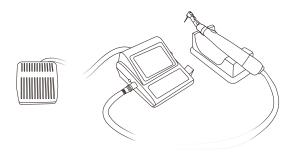
M3: Reciprocating rotation function, hold down the foot switch or press the handle, the file starts to reciprocating rotation, rotating situation for the reverse 150°, forward 30°, the speed of about 300 RPM. Loosen the foot switch or press the handle button, the file will stop running.
