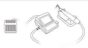
**M2:** Single root canal expanded function, hold down the foot switch or press the handle button, the file will rotate; when the file arrived at the setting torque, the file will automatically reverse. When the torque reduces, the file will recover forward. Loosen the foot switch or press the handle button, the file stops rotating.
